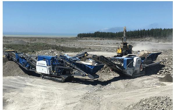
**Figure 35 - Mobile crushing and screening**
