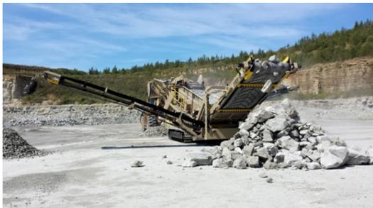
**Figure 34 - Mobile screening plant**
